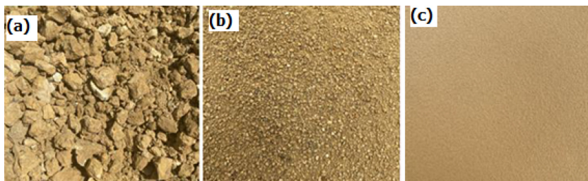
Fig. 1. Samples of bentonite (a) Bentonite ore; (b) Bentonite powder; (c) Purification bentonite using the hydrocyclone method.
