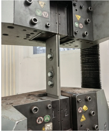
Fig. 4. Tensile testing of specimens in a tensile testing machine
