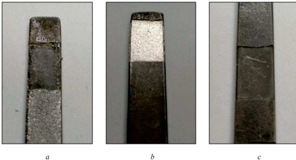
Fig. 6. The surface of specimens as a result of electrochemical etching of specimens made of 3Cr2W8V steel after CTT:
