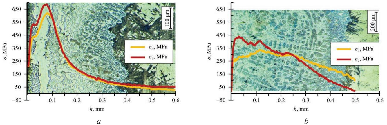
Fig. 8. Diagrams of residual stresses in a plate made of  $5CrNiMo$  steel at a treatment temperature:
