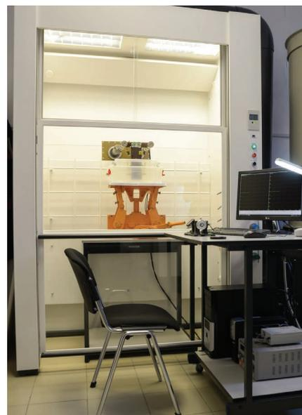
Fig. 2. Installation for measuring residual stresses by mechanical method (UDION-2)
