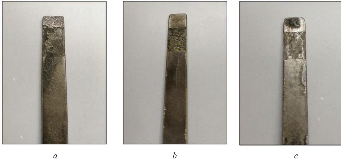
Fig. 4. The surface of specimens as a result of chemical etching of specimens made of 3Cr2W8V steel after CTT:
