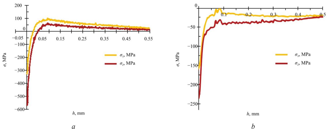
Fig. 7. Diagrams of residual stresses in a plate:
