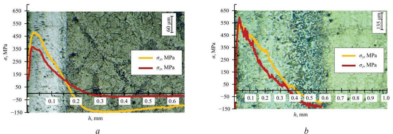
Fig. 9. Diagrams of residual stresses in a plate made of  $3Cr2W8V$  steel at a processing temperature:
