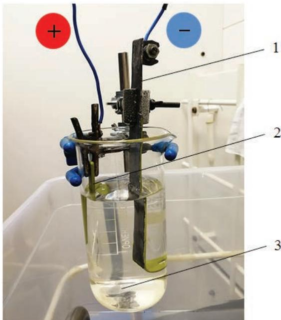
Fig. 5. Electrochemical cell for testing the process of anodic dissolution:
