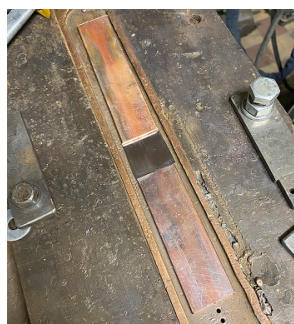
Fig. 2. GTAW welding fixture ( a ), specimens for mechanical testing ( b ) and microhardness testing specimens ( c ) of the welded joint of Ti-Al-Nb-(Zr, Mo)-Si alloy
