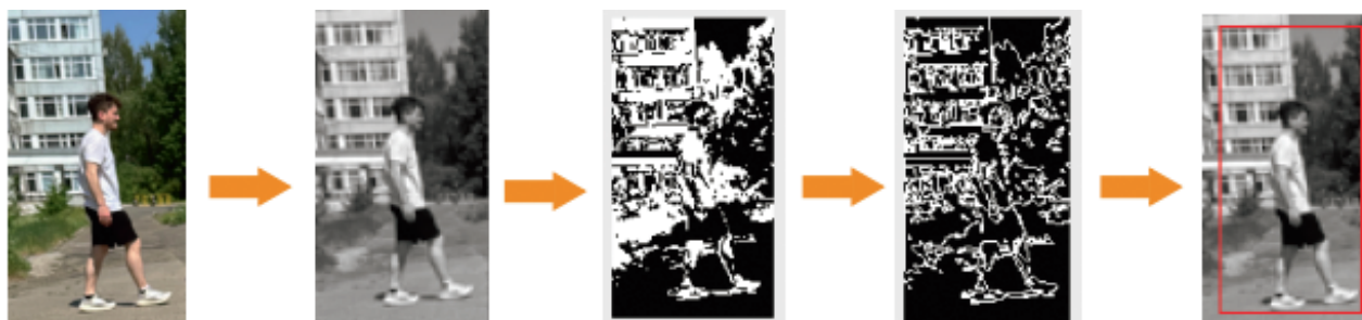
Fig. 8. The principle of operation of the algorithm for recognizing a person in an image.
