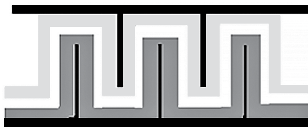
Fig. 2. 3D design with interdigital arrays of electrodes.
