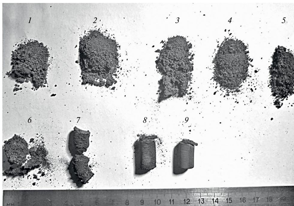
Fig. 6. Photograph of samples of combustion products of activated mixtures 60\%(\text{Ti}+2\text{B})+40\%(\text{Ti}+\text{C})+x(5\text{Me}) , x= : 1–0%, 2–10%, 3–20%, 4–30%, 5–40%, 6–50%, 7–60%, 8–70%, 9–80% wt. %
