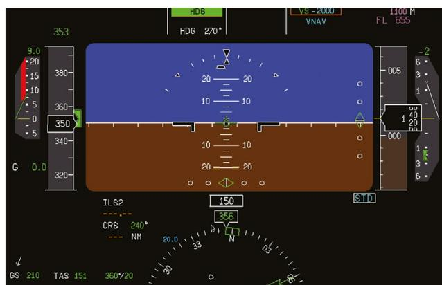
Рис. 4. Primary Flight Display MC\_PFD.
