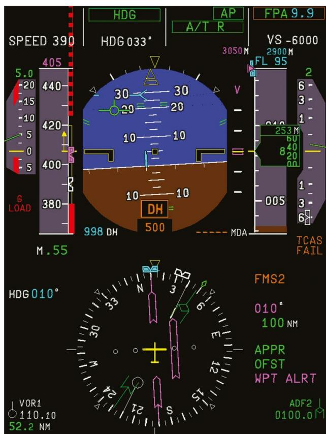
Рис. 3. Primary Flight Display SS\_PFD.
