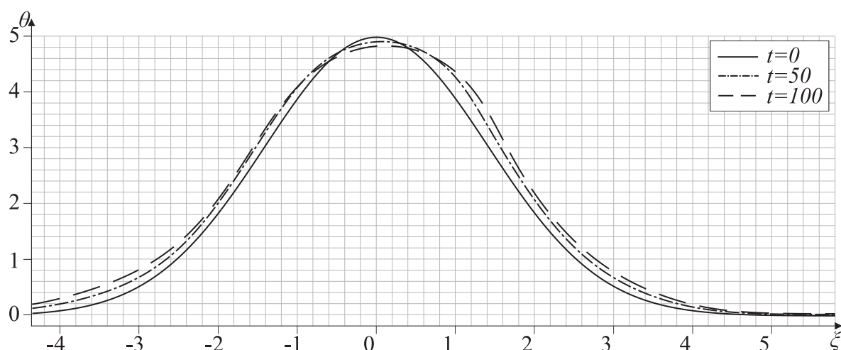
Фиг. 5. Намерзание, T_{\text{ice}} = -5^\circ\text{C} , T_{\text{water}} = -1^\circ\text{C} .
